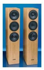
The Solitude set-up combines the direct, highly precise sound reproduction of the B 200 6 Ohm wide-range speaker with the dynamic bass of two GF 200 2 x 4 Ohm. The B 200 6 Ohm is fitted in a completely enclosed, heavily damped compartment. The two GF 200 2 x 4 Ohm woofers are mounted in a voluminous cabinet with a generously dimensioned bass reflex tube. Owing to the very low-frequency separation, Solitude is, in effect, a wide-range speaker with a subwoofer.
